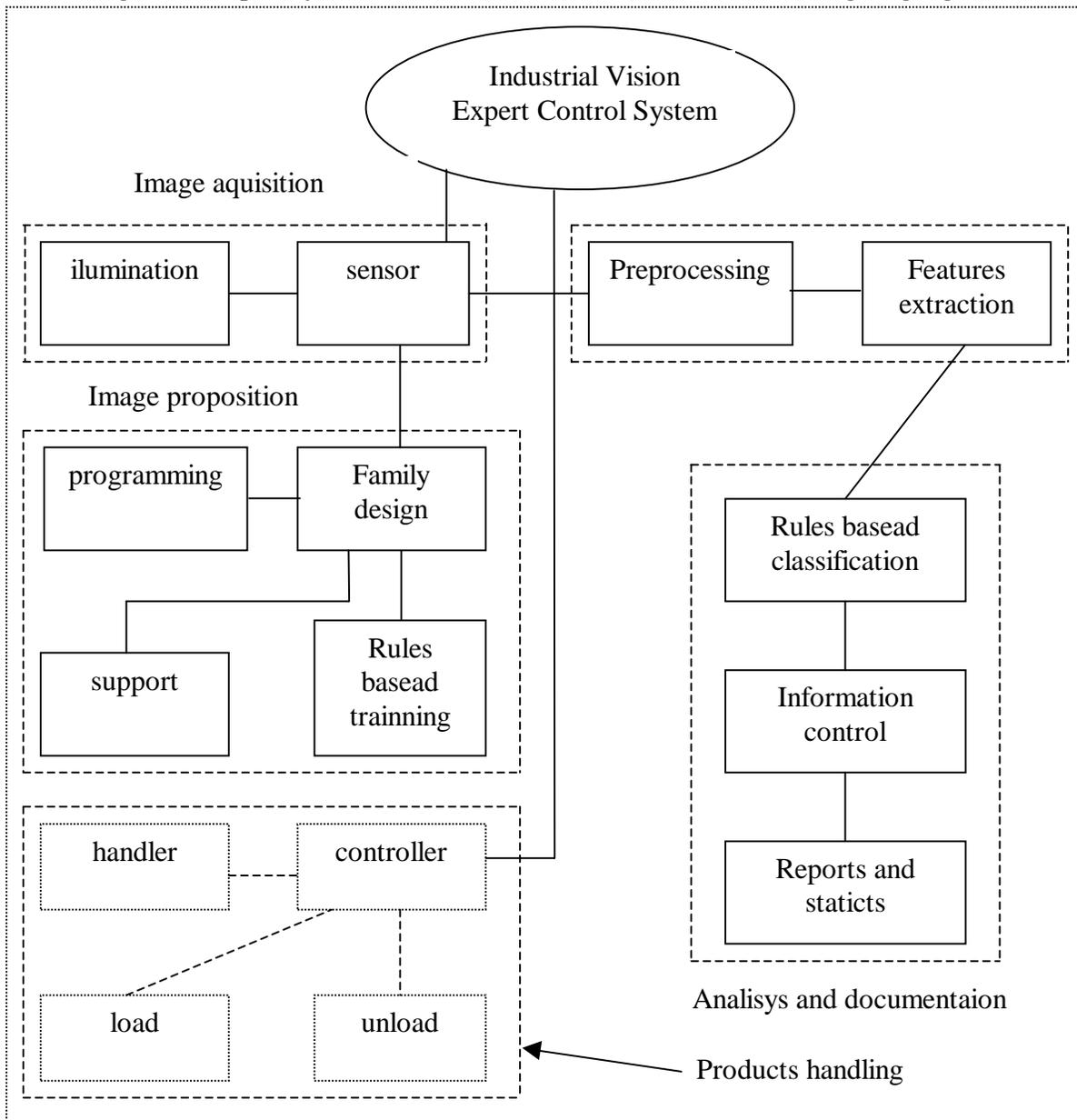
**Figure 3 - Block diagram for the control system**
